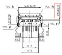
**2.** The gap increasing between shell and PCB is to avoid short circuit and raise safety factor, and stand-off area change of housing is to avoid soldering overlapping.
