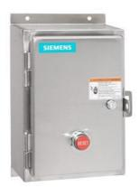
Non-reversing motor starter, Size 1, Single phase full voltage, Solid-state overload relay, OLR amp range 5.5-22A, Non-combination type, Encl. type 4X 304 S. Steel, Water/dust tight noncorrosive, Standard width enclosure
