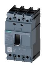
circuit breaker 3VA5 UL frame 125 breaking capacity class H 65kA @ 480 V 3-pole, line protection TM210, FTFM, In=40A overload protection Ir=40A fixed short-circuit protection Ii=10 x In UL489 SB (naval), 50 deg. cel. nut keeper kit on both sides
