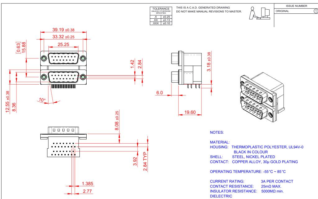
WITHSTANDING VOLTAGE: 1000V AC rms
