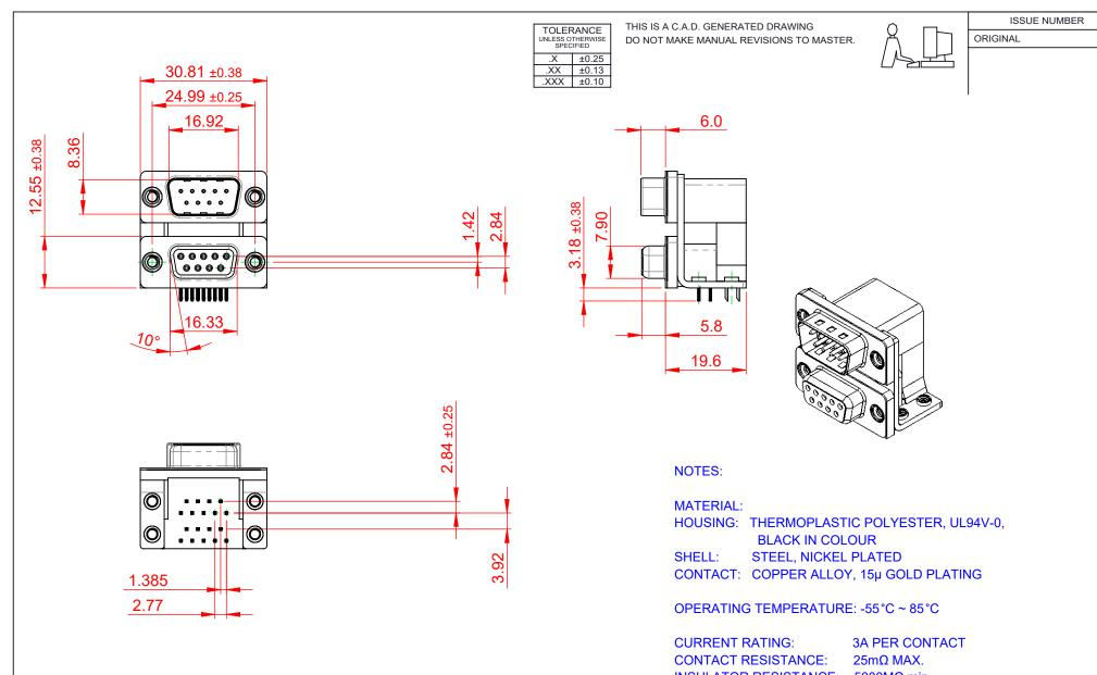
INSULATOR RESISTANCE: 5000MΩ min. DIELECTRIC WITHSTANDING VOLTAGE: 1000V AC rms (1)
