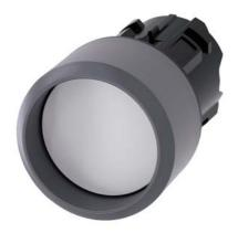
Pushbutton, 22 mm, round, plastic with metal front ring, white, Front ring, raised momentary contact type, with laser labeling, inscription or symbol Customer-specific selection with SIRIUS ACT configurator (CIN)
