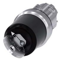
Key-operated switch IKON, 22 mm, round, metal, shiny, lock number 360012K1, with 2 keys, 2 switch positions O-I, latching, actuating angle 90°, 10:30h/13:30h, key removal O+I, with laser labeling, lower case
