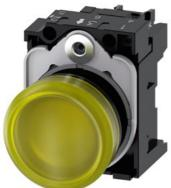
Indicator lights, 22 mm, round, plastic, yellow, lens, smooth, with holder, LED module with integrated LED 110 V AC, screw terminal, with laser labeling, inscription or symbol Customer-specific selection with SIRIUS ACT configurator (CIN)
