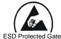
ESD Protected Gate
