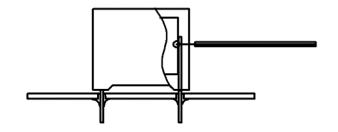
Temperature monitored inside the capacitor.
