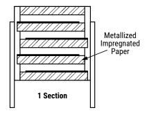
Film Capacitors – AC Line EMI Suppression and RC Networks PME278, Metallized Impregnated Paper, Class X1, 440 VAC
