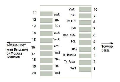
Pin-out of connector Block on Host board
