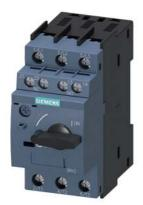
Circuit breaker size S00 for transformer protection A-release 0.9...1.25 A N-release 26 A screw terminal Standard switching capacity with transverse auxiliary switches 1 NO+1 NC  $\,$
