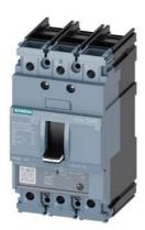
circuit breaker 3VA5 UL frame 125 breaking capacity class M 35kA @ 480 V 3-pole, line protection TM230, FTAM, In=70A overload protection Ir=70A fixed short-circuit protection Ii=5...10 x In UL489 SB (naval), 50 deg. cel. cable connection on both sides
