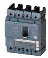
circuit breaker 3VA5 UL frame 250 breaking capacity class H 65kA @ 480V 4-pole, line protection TM210, FTFM, In=200A overload protection Ir=200A fixed short-circuit protection li=10 x In N conductor protection 100% without connection
