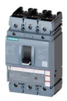
circuit breaker 3VA5 UL frame 250 breaking capacity class H 65kA @ 480 V 3-pole, line protection TM230, FTAM, In=80A overload protection Ir=80A fixed short-circuit protection li=5...10 x In cable connection on both sides
