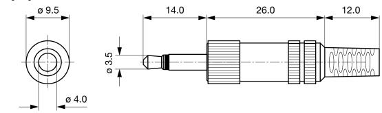
Cable diameter max. 4.0 mm
