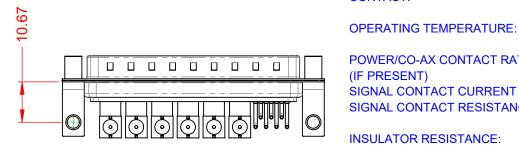
POWER/CO-AX CONTACT RATING: (IF PRESENT) SIGNAL CONTACT CURRENT RATING: 5A PER CONTACT SIGNAL CONTACT RESISTANCE:  $10m\Omega$  MAX. **INSULATOR RESISTANCE:** 5000MΩ min.
