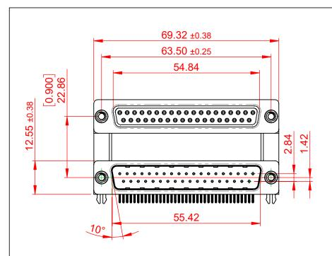
THIS IS A C.A.D. GENERATED DRAWING TOLERANCE UNLESS OTHERWISE SPECIFIED DO NOT MAKE MANUAL REVISIONS TO MASTER. .X ±0.25 .XX ±0.13 .XXX ±0.10 6 5.8 ų, 6.0 **3.18** ±0.38 19.6
