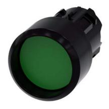
Pushbutton, 22 mm, round, plastic, green, Front ring, raised momentary contact type, with laser labeling, symbol number according to, ISO 7000 or IEC 60417
