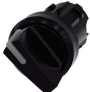
Illuminable selector switch, 22 mm, round, plastic, black, Selector switch short, 2 switch positions O-I, latching, actuating angle 90°, 10:30 /13:30, Z=50-unit packaging
