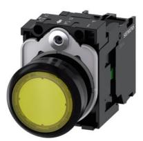
Illuminated pushbutton, 22 mm, round, plastic, yellow, pushbutton, flat, momentary contact type, with holder, 1NO, LED module with integrated LED 110 V AC, screw terminal, with laser labeling, inscription or symbol Customer-specific selection with SIRIUS ACT configurator (CIN)
