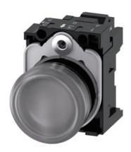
Indicator lights, 22 mm, round, plastic, clear, lens, smooth, with holder, LED module, with integrated LED 110 V AC, spring-type terminal, with laser labeling, inscription or symbol Customer-specific selection with SIRIUS ACT configurator (CIN)
