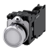
Illuminated pushbutton, 22 mm, round, metal, shiny, white, pushbutton, flat, momentary contact type, with holder, 1 NO+1 NC, LED module with integrated LED 24 V AC/DC, spring-type terminal, with laser labeling, lower case
