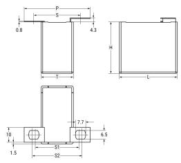
**General Information** Series C4BS Dielectric Metallized Polypropylene Style Radial IGBT Circuit Features RoHS Yes Lead Flat Tabs AEC-Q200 No **Component Weight** 58.33 g KEMET Style E Tabs. Miscellaneous
