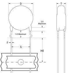
position of Lead Spacing (S) and Width (V) is critical in straight lead capacitors.
