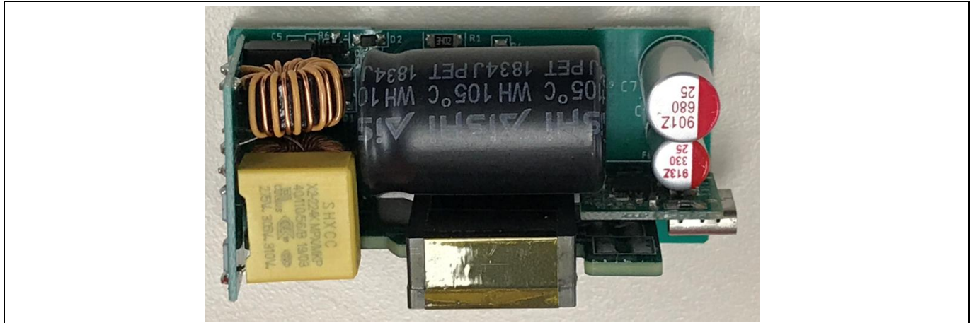
Figure 1 REF_XDPS21071_45W1 FFR ZVS Flyback converter (top view)
