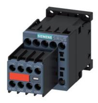
Power contactor, AC-3 12 A, 5.5~kW / 400~V 2 NO + 2 NC, 24~V DC with diode integrated 3-pole, Size S00 Screw terminal Captive auxiliary switch
