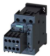
power contactor, AC-3 17 A, 7.5 kW / 400 V 2 NO + 2 NC, 110 V AC, 50 Hz, 3-pole, Size S0 screw terminal Removable auxiliary switch
