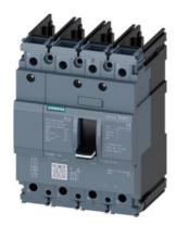
circuit breaker 3VA5 UL frame 125 breaking capacity class S 25kA @ 480V 4-pole, line protection TM210, FTFM, In=60A overload protection Ir=60A fixed short-circuit protection Ii=10 x In N conductor unprotected without connection
