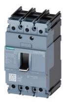
circuit breaker 3VA5 UL frame 125 breaking capacity class S 25kA @ 480 V 3-pole, line protection TM210, FTFM, In=90A overload protection Ir=90A fixed short-circuit protection Ii=10 x In UL489 SB (naval), 50 deg. cel. cable connection on both sides
