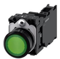
Illuminated pushbutton, 22 mm, round, plastic, green, pushbutton, flat, momentary contact type, with holder, 1 NO+1 NC, LED module with integrated LED 24 V AC/DC, spring-type terminal, with laser labeling, upper case and lower case, always upper case at beginning of line
