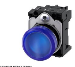
Indicator lights, 22 mm, round, metal, shiny, blue, lens, smooth, with holder, LED module with integrated LED 24 V AC/DC, screw terminal, with laser labeling, inscription or symbol Customer-specific selection with SIRIUS ACT configurator (CIN)
