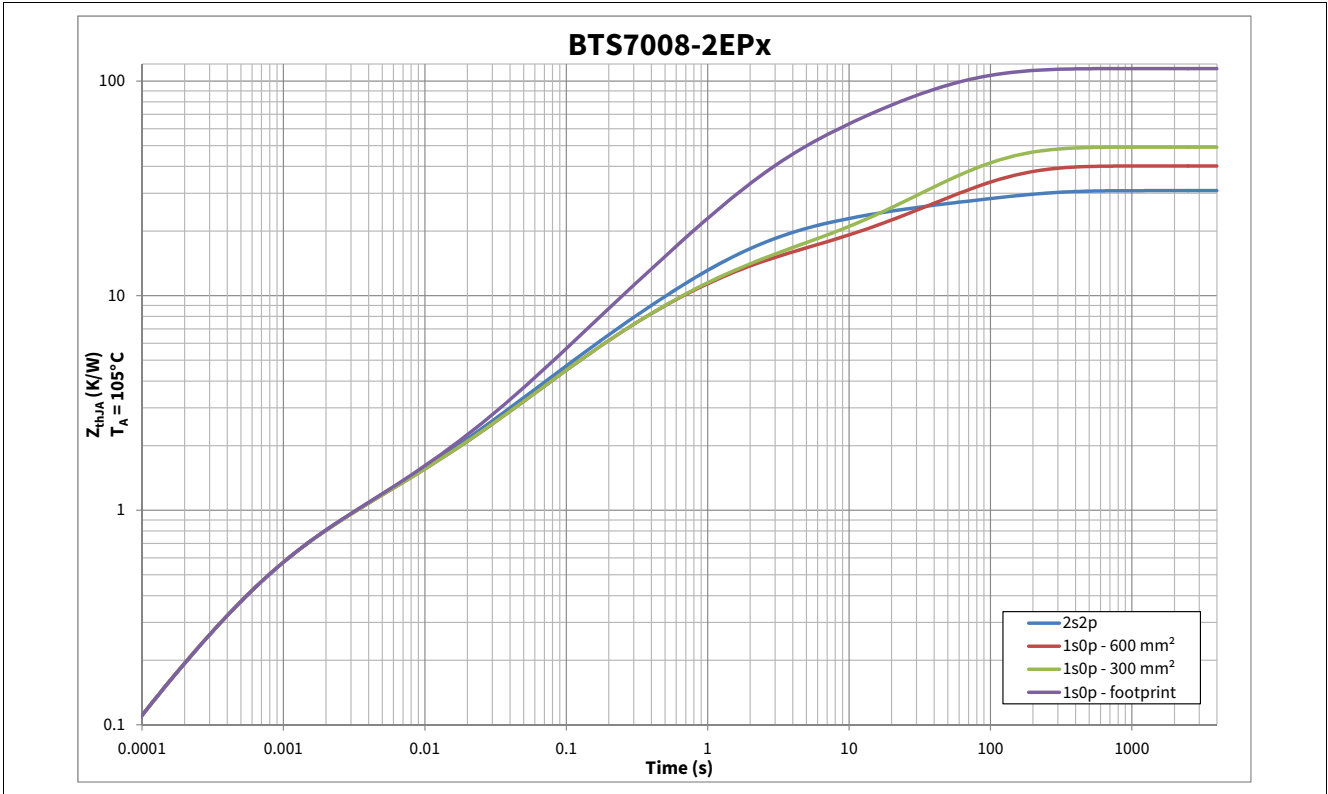
Figure 9 Typical Thermal Impedance. PCB setup according Chapter 4.4.1
