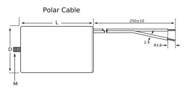
General Information Series C28 Dielectric Film/Foil Polypropylene Style Plastic Case and Cover, Ultra Sonically Welded Description Ultra Sonically Welded Seal, Safety Class S3, UL\_94 V0 Disk **Features** RoHS Yes Termination Tin Copper Cables UL, VDE, UL (Construction Only), UL\_94 VO Disk Qualifications AEC-Q200 Component 27 g Weight
