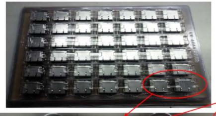
Old top tray: the holder of the top tray is close to the shield pins and will have a chance to have the shield pin deformed by pressure.
