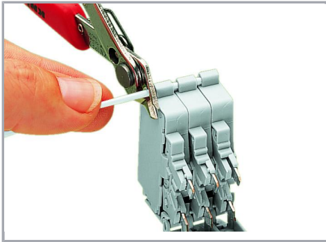
Ganging several fuse holders with an interlocking link (example shows 8 mm wide terminal blocks).
