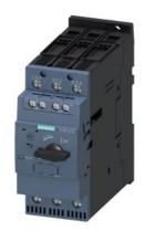
Circuit breaker size S2 for motor protection, CLASS 10 A-release 70...80 A N-release 1040 A screw terminal increased switching capacity with transverse auxiliary switches 1 NO+1 NC
