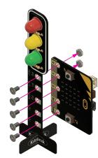
**Connection:** x5 M3 countersunk screws allow the user to bolt the STOP:bit onto the BBC micro:bit. Crocodile clips also can be used between the pads on the STOP:bit and the matching pads on the BBC micro:bit.
