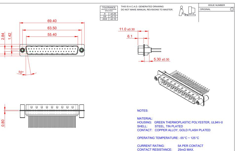
DIELECTRIC WITHSTANDING VOLTAGE: 1000V AC rms
