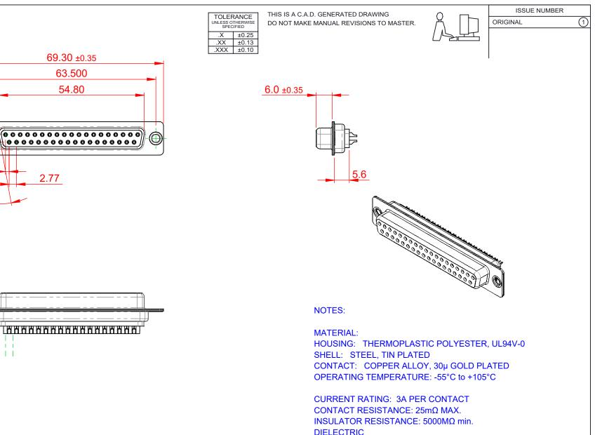
WITHSTANDING VOLTAGE: 1000V AC rms
