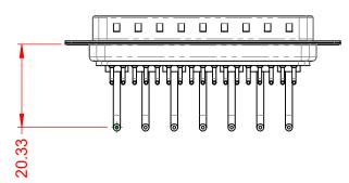
POWER/CO-AX CONTACT RATING:10A (CURRENT)(IF PRESENT)SIGNAL CONTACT CURRENT RATING:5A PER CONTACTSIGNAL CONTACT RESISTANCE:10mΩ MAX.INSULATOR RESISTANCE:5000MΩ min.
