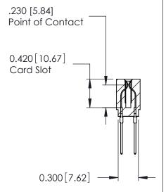
ACAD REFERENCE NO. 725-ENG MASTER 725 Series Ultra-Mate Card Edge Connector - Press Fit SEGAHON:3A:9A DRAWN: J.LEE Part Number: 725-040-545-201 CHECKED: DATE: SCALE: **EDAC INC** SHEET 1 OF 1 THESE DRAWINGS AND SPECIFICATIONS ARE THE PROPERTY OF EDAC INC.,AND TORONTO, ONTARIO SHALL NOT BE REPRODUCED, OR COPIED DRAWING NUMBER **ISSUE** CANADA OR USED AS THE BASIS FOR THE 725-ENG MASTER MANUFACTURE OR SALE OF APPARATUS YOUR CONNECTION TO QUALITY & SERVICE WITHOUT WRITTEN PERMISSION.
