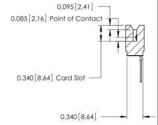
ACAD REFERENCE NO. 746 Series Ultra-Mate Card Edge Connector - Press Fit DRAWN: J.LEE Part Number: 746-025-540-506 CHECKED: **EDAC INC** SCALE: THESE DRAWINGS AND SPECIFICATIONS ARE THE PROPERTY OF EDAC INC.,AND TORONTO, ONTARIO SHALL NOT BE REPRODUCED, OR COPIED DRAWING NUMBER CANADA OR USED AS THE BASIS FOR THE 746-ENG MASTER MANUFACTURE OR SALE OF APPARATUS YOUR CONNECTION TO QUALITY & SERVICE WITHOUT WRITTEN PERMISSION.
