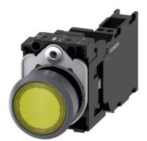
Illuminated pushbutton, 22 mm, round, plastic with metal front ring, yellow, pushbutton, flat, momentary contact type, with holder, 1 NO+1 NC, LED module with integrated LED 24 V AC/DC, spring-type terminal, with laser labeling, lower case
