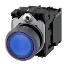
Illuminated pushbutton, 22 mm, round, plastic with metal front ring, blue, pushbutton, flat, momentary contact type, with holder, 1NO, LED module with integrated LED 230 V AC, screw terminal, with laser labeling, inscription or symbol Customer-specific selection with SIRIUS ACT configurator (CIN)
