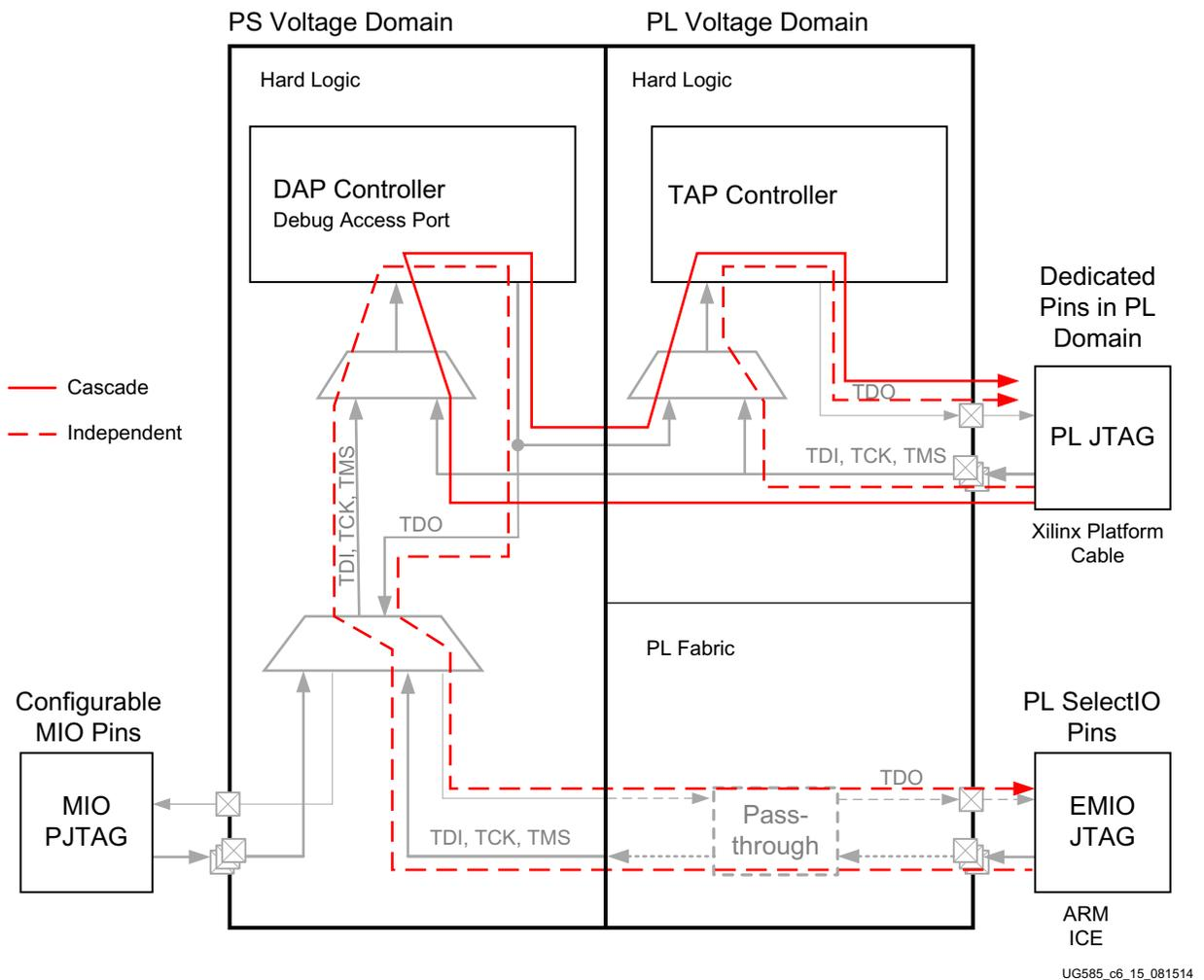
Figure 6-7: PS Cascade and Independent JTAG Chain Diagram
