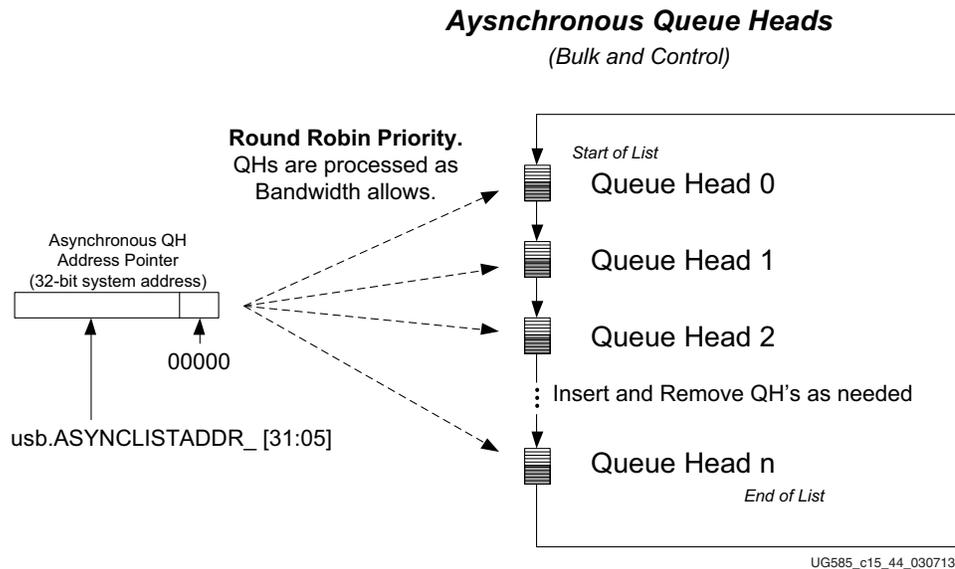
Figure 15-16: USB Host Controller Asynchronous Schedule Organization
