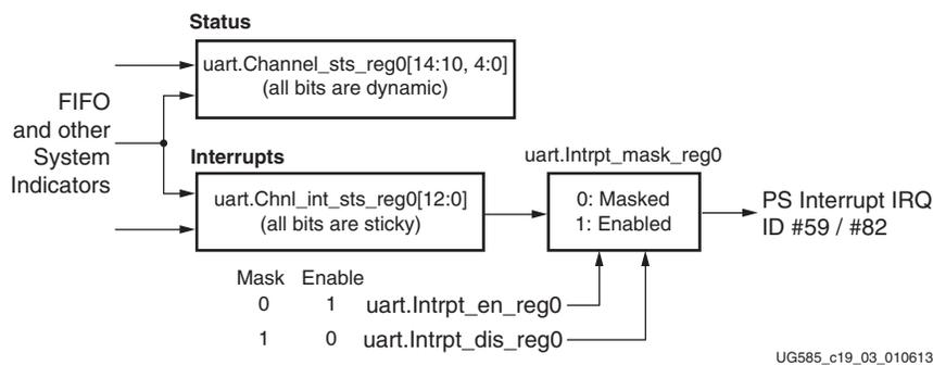
Figure 19-8: Interrupts and Status Signals
