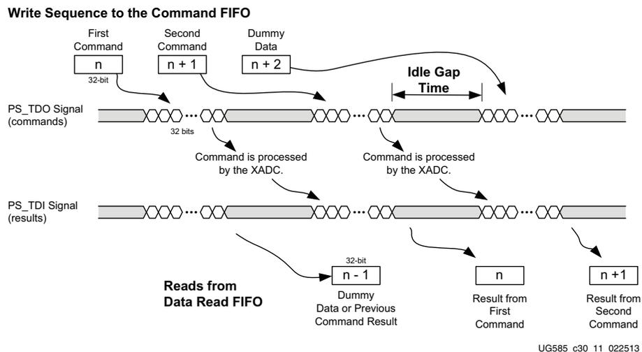
Figure 30-3: XADC PS-XADC Interface Event Timing Diagram
