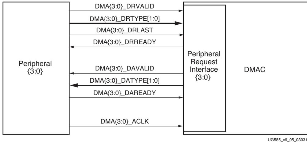
Figure 9-4: DMAC PL Peripheral Request Interface Request/Acknowledge Signals
