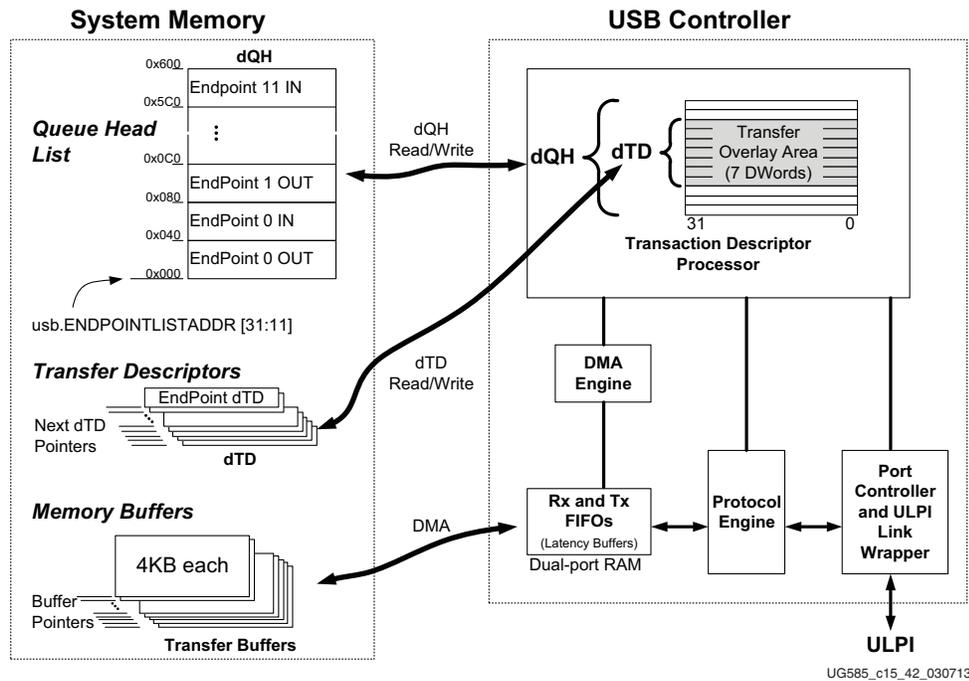
Figure 15-14: USB Device Descriptor and Data Flow
