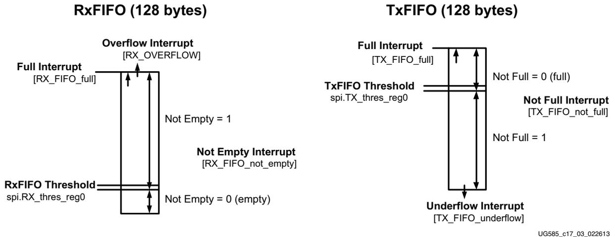
Figure 17-3: SPI Rx and Tx FIFO Interrupts
