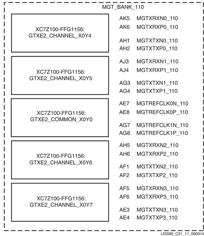
Figure 21-11: XC7Z100-FFG1156, MGT Bank 110 Package Placement Diagram
