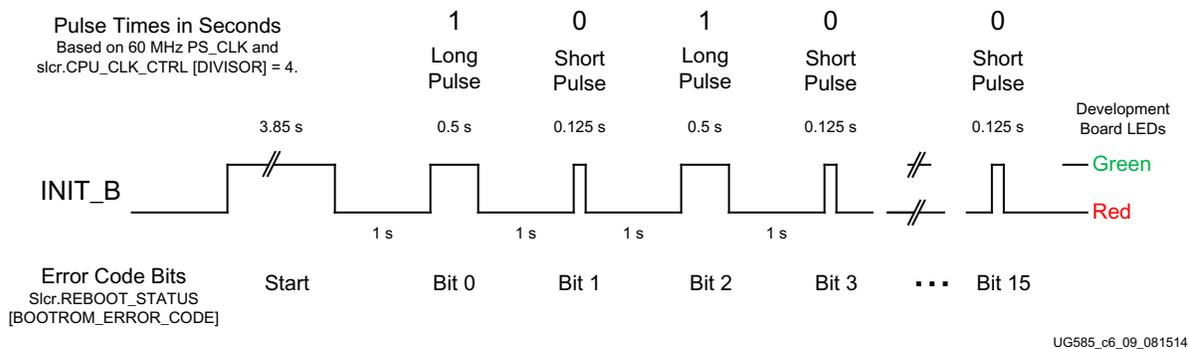
Figure 6-10: Error Code INIT\_B Bit Waveform Example
