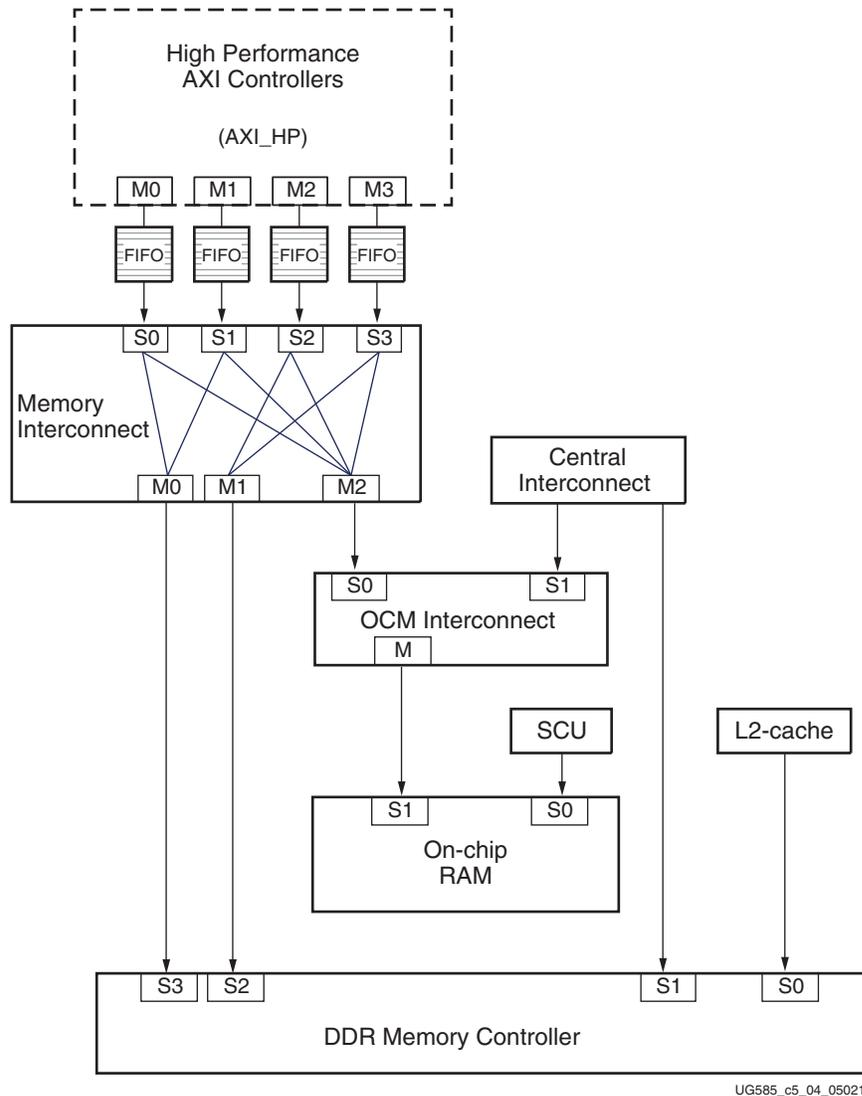
Figure 5-4: High Performance (AXI\_HP) Connectivity
