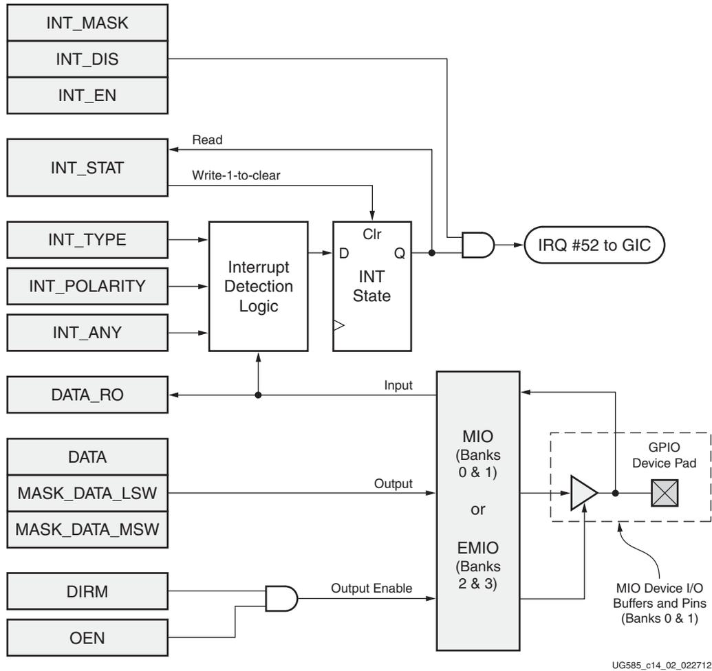
Figure 14-2: GPIO Channel
