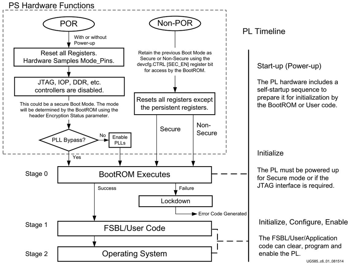
Figure 6-1: PS/PL Boot Process for Hardware and Software
