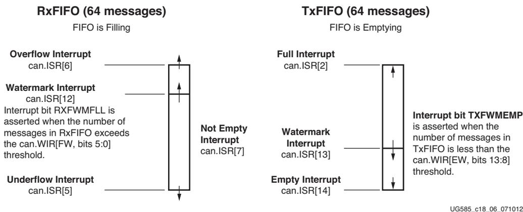
Figure 18-4: CAN RxFIFO and TxFIFO Watermark Interrupts
