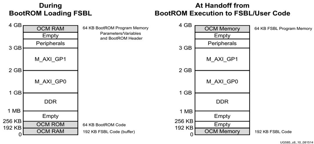
Figure 6-11: System Memory Map During BootROM Execution
