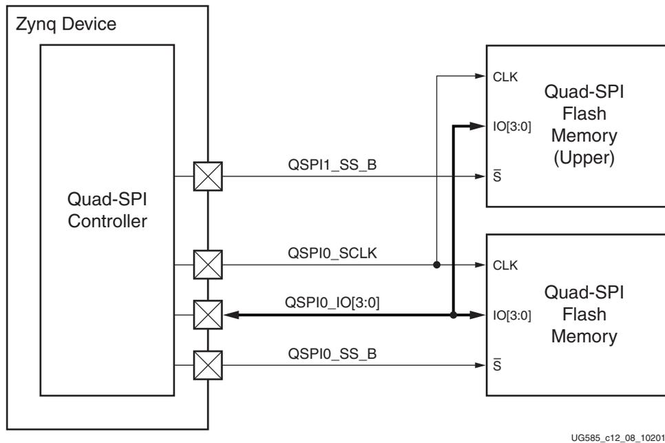
Figure 12-7: Quad-SPI Dual SS 4-bit Stacked I/O
