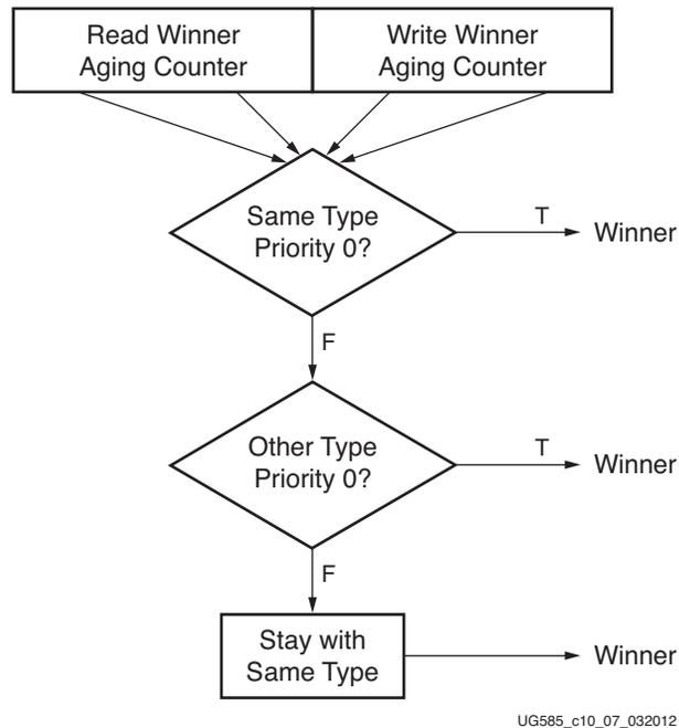
Figure 10-7: Stage 2 – Read Versus Write
