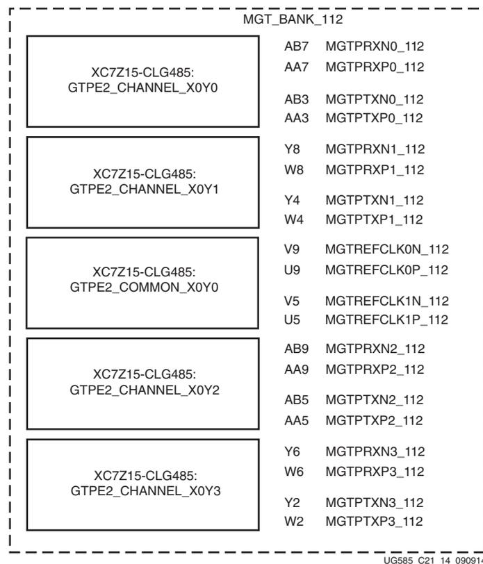
Figure 21-14: XC7Z012S-CLG485 and XC7Z015-CLG485 Package Placement Diagram
