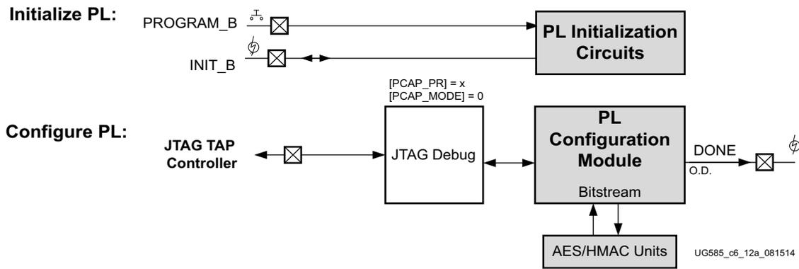
Figure 6-20: PL Initialization and Configuration Using User-JTAG
