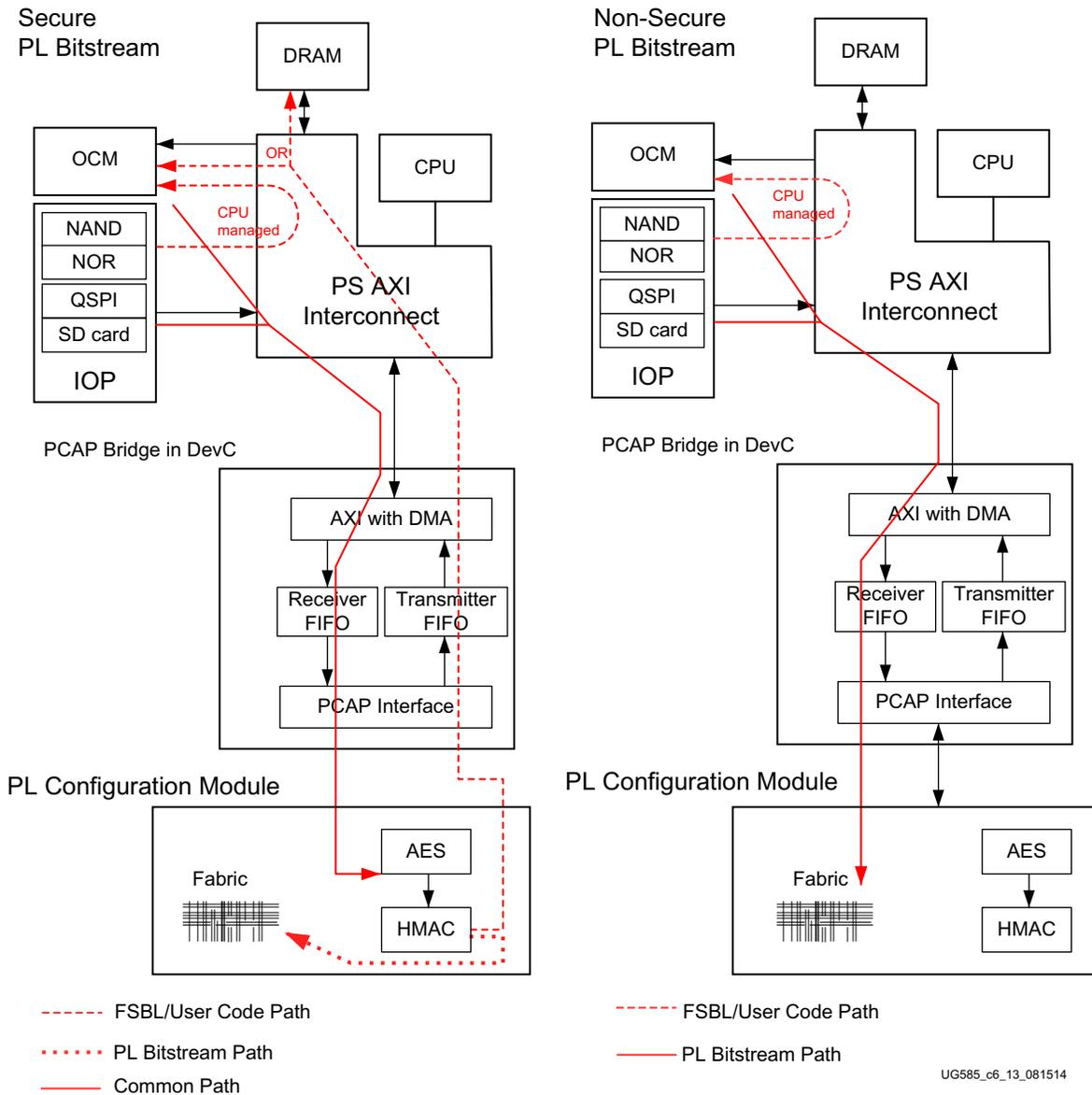
Figure 6-18: Non-Secure and Secure PL Bitstream Path Diagrams
