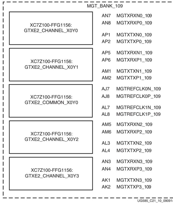
Figure 21-10: XC7Z100-FFG1156, MGT Bank 109 Package Placement Diagram
