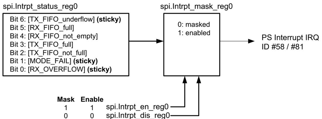
Figure 17-4: SPI Interrupt Register Bits, Logic Flow
