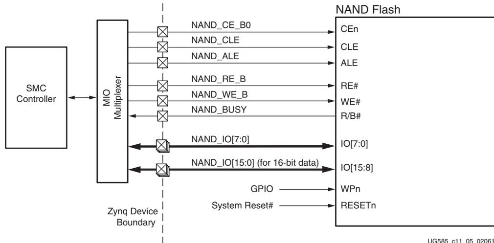
Figure 11-5: NAND Flash Device Wiring Diagram
