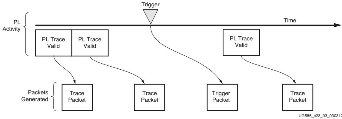
Figure 23-3: Packet Generation, No Cycle Count Case
