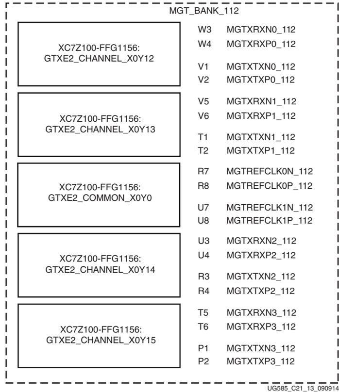
Figure 21-13: XC7Z100-FFG1156, MGT Bank 112 Package Placement Diagram
