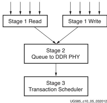
Figure 10-5: DDRC Arbitration
