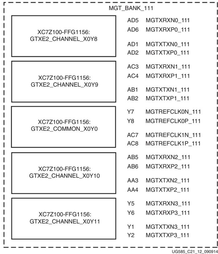
Figure 21-12: XC7Z100-FFG1156, MGT Bank 111 Package Placement Diagram
