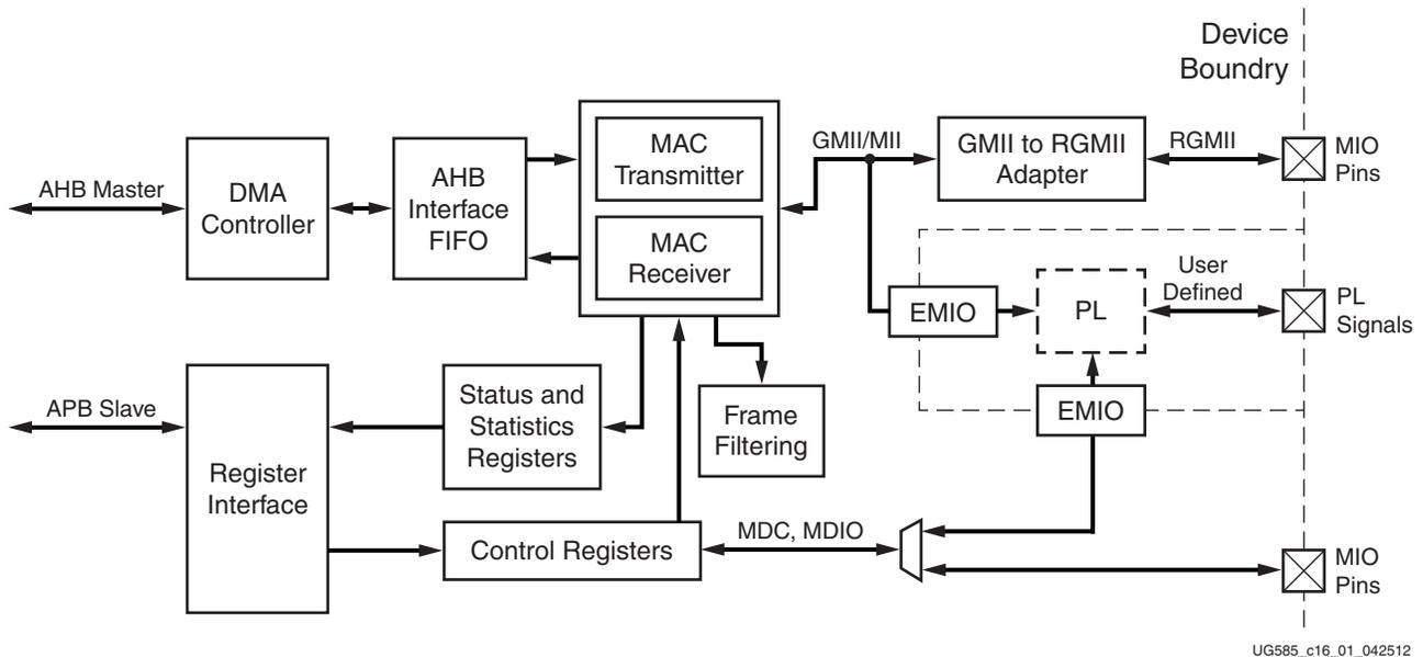
Figure 16-1: Ethernet Controller
