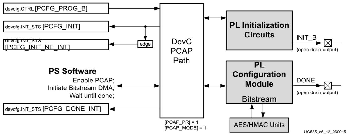
Figure 6-12: PCAP Path for PL Initialization and Configuration
