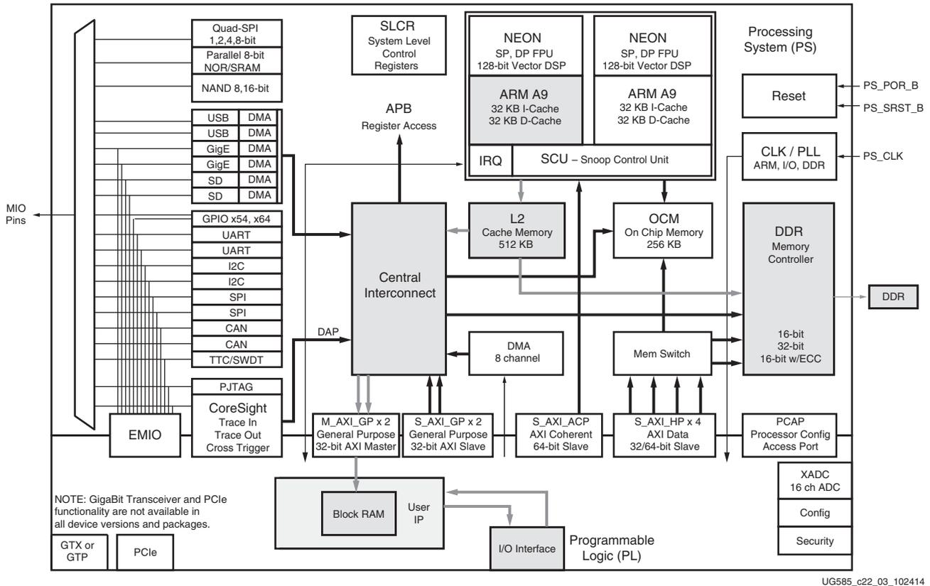
Figure 22-1: Example Cortex-A9 PL Data Movement Topology
