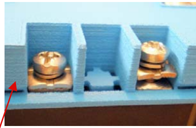
Connexions de commande M4 M4 control connections
