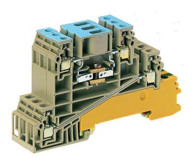
Three-wire installation terminal, Screw connection, Mounting type: Mounting rail TS 35/7.5, Rated cross-section: 2.5 mm², Width: 18 mm, Colour: Beige
