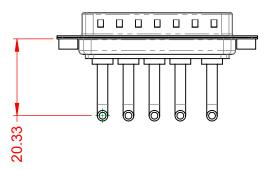
20A (CURRENT) POWER/CO-AX CONTACT RATING: (IF PRESENT) SIGNAL CONTACT CURRENT RATING: 5A PER CONTACT SIGNAL CONTACT RESISTANCE:  $10m\Omega$  MAX. INSULATOR RESISTANCE:
