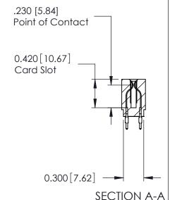
725 Series Ultra-Mate Card Edge Connector - Press Fit ACAD REFERENCE NO.
